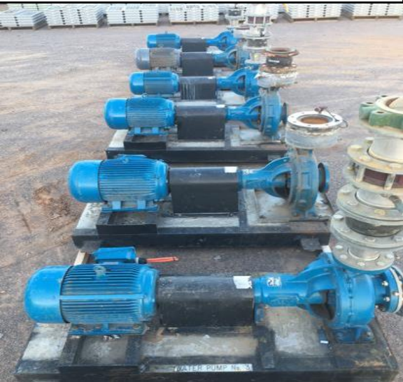
Image 4. Mt Freda Leach Vat pumps being assembled
