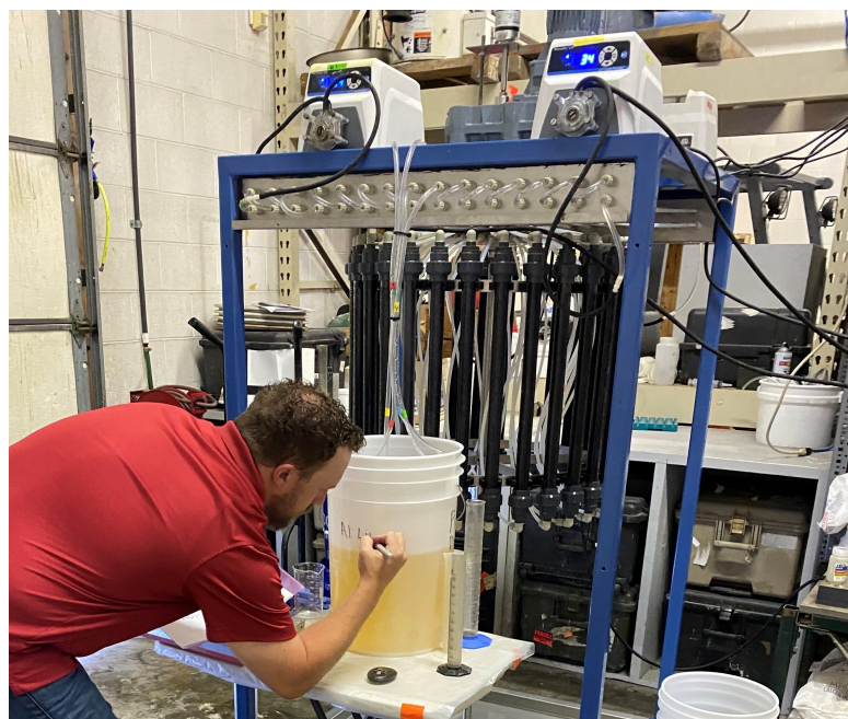
Figure 1: Small-scale pilot plant using water to wash off lithium from resin.
