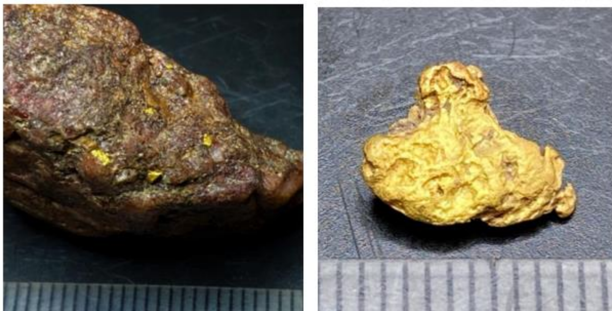
Figure 4 - Toolebuc gold samples. Left: Coarse (~1mm) gold grains peppered through host rock. Right: 10mm sized gold nugget. Scale marked at 1mm intervals in both photos.
