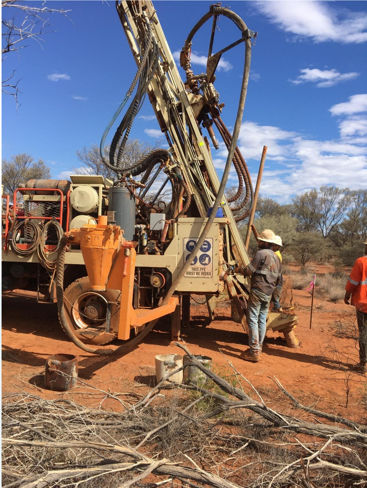
Figure 3. Aircore drilling of regional targets at Youanmi is underway.
