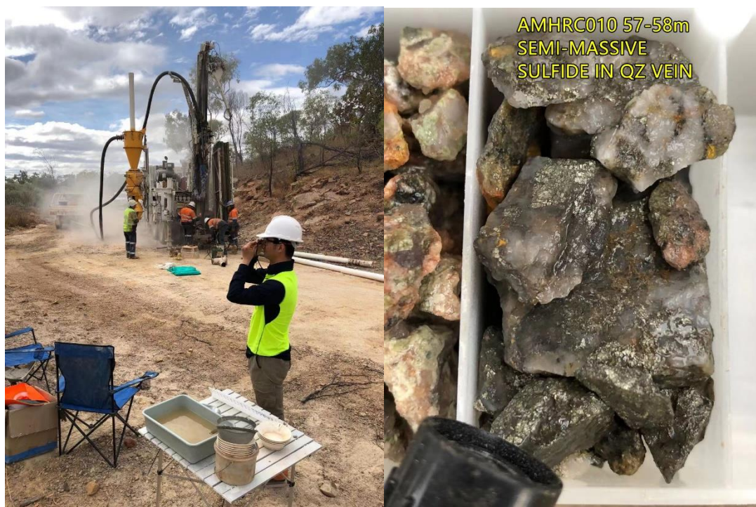
Plate 1. Drilling at Mt Hogan and a pyritic quartz interval from the drilling campaign.
