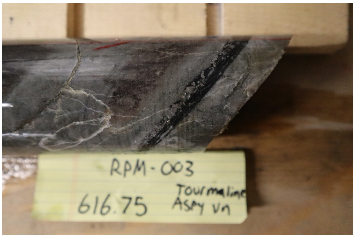
Figure 9: RPM-003 – Tourmaline-Arsenopyrite vein in hornfels
