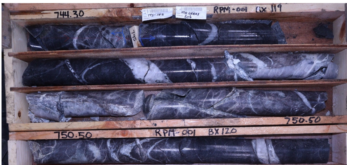
Figure 2: RPM-001- Strong quartz-carbonate veining with tourmaline and minor sulfide
