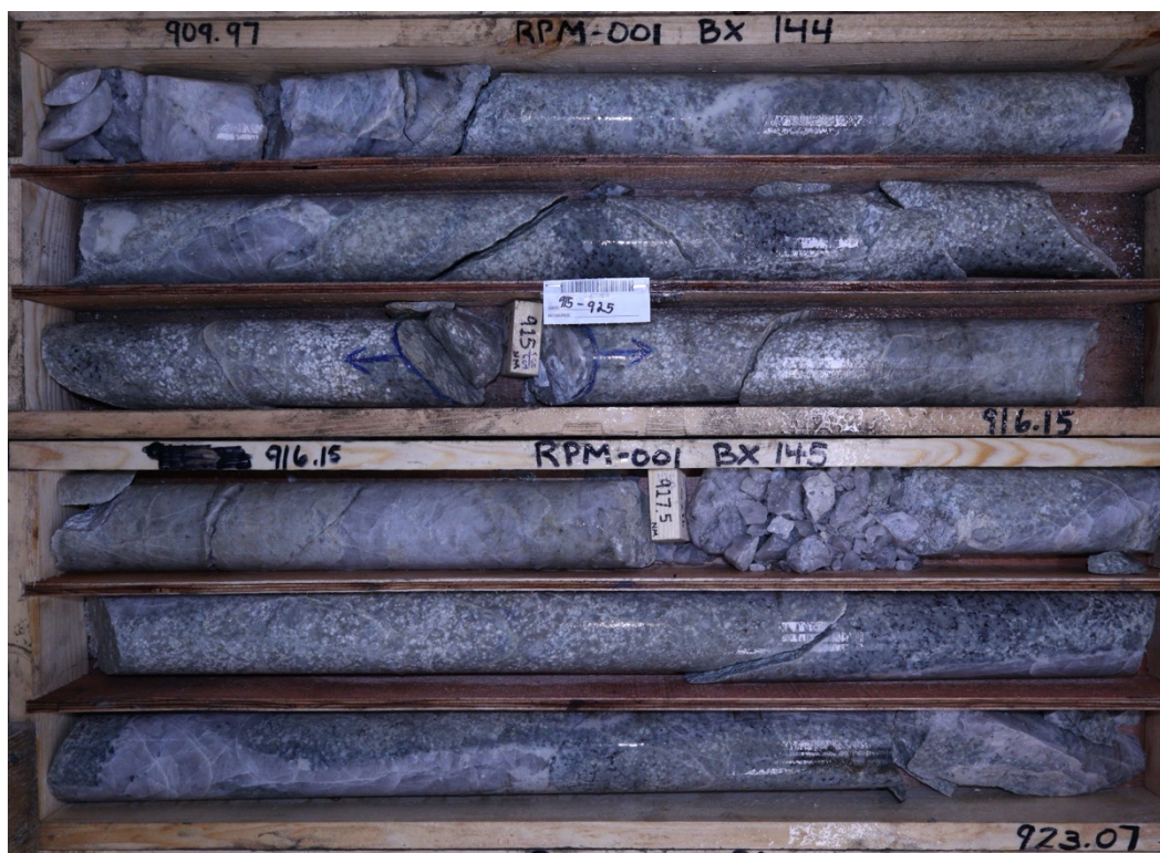
Figure 4: RPM-001 - Quartz veining with minor sulfide in phyllic altered granitic intrusive
