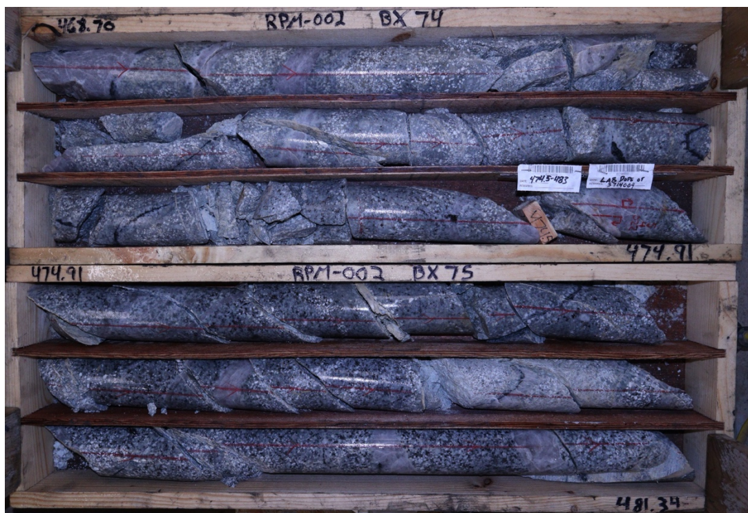
Figure 3: RPM-002 - Typical low sulfide quartz-tourmaline-sulfide veining in phyllic altered granitic intrusive
