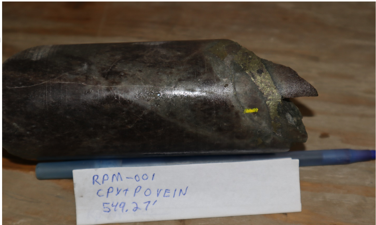
Figure 6: RPM-001 - Chalcopyrite-pyrrhotite vein in hornfels
