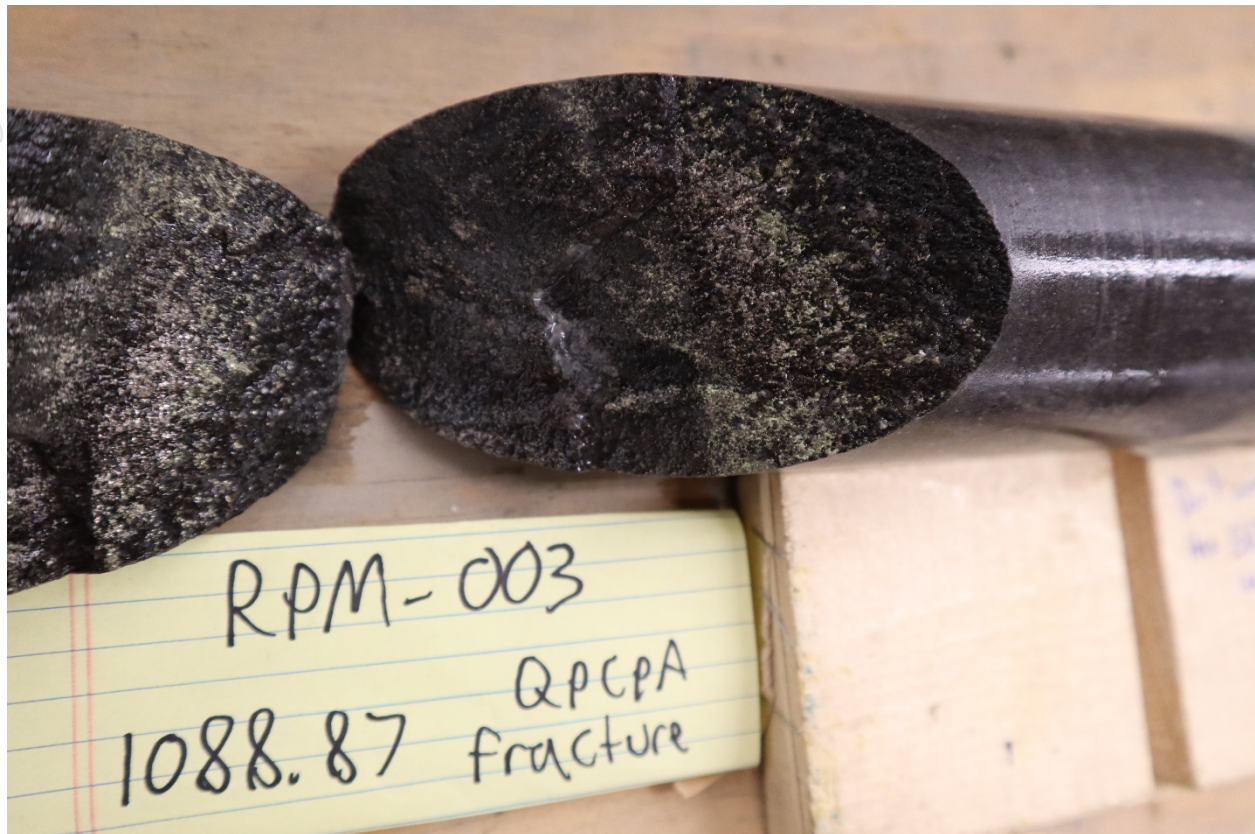
Figure 8: RPM-003 Pyrite-Chalcopyrite mineralisation in hornfels
