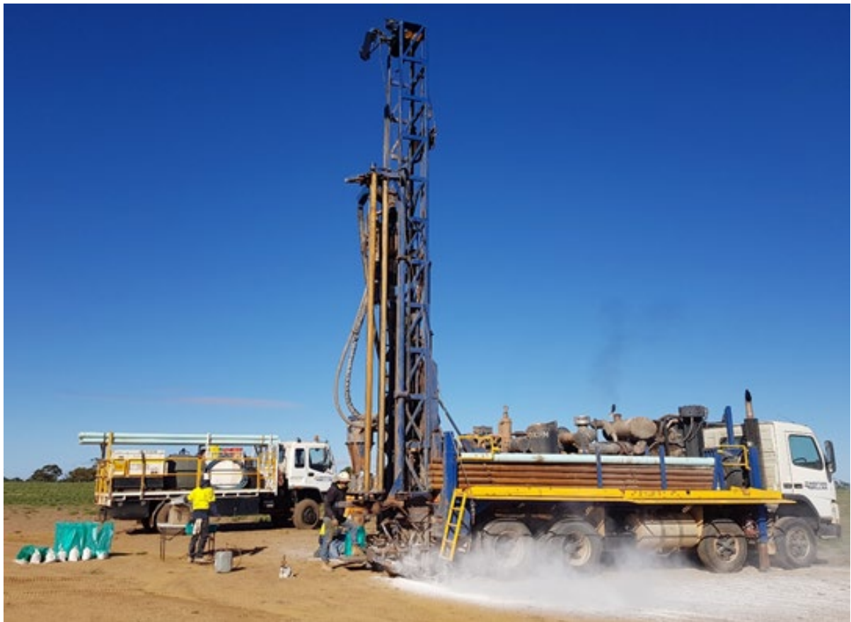
Figure 2: Drilling bright white kaolin at shallow depth (Tampu, May 2021)
