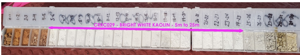
Figure 4: Drillhole CRRC029 with bright white kaolin from 5m to 25m (20m intercept)
