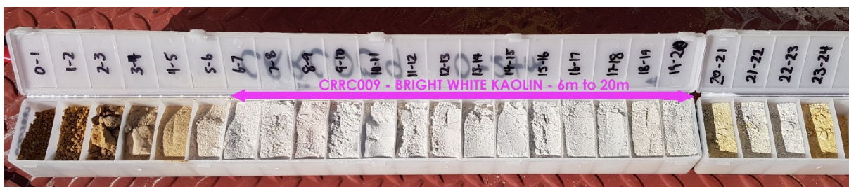
Figure 5: Drillhole CRRC009 with bright white kaolin from 6m to 20m (14m intercept)
