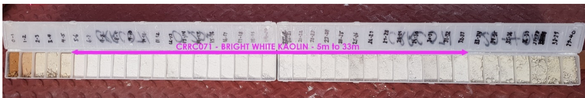
Figure 3: Drillhole CRRC071 with bright white kaolin from 5m to 33m (28m intercept)
