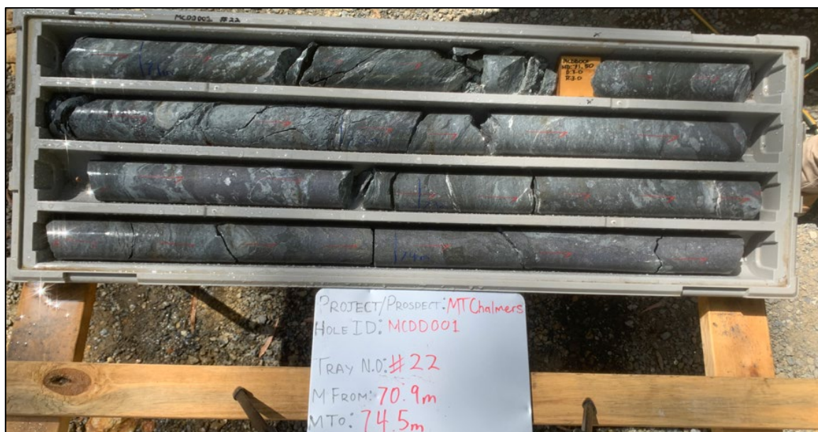
Figure 8: DDH001 laminated semi-massive sulphides including galena, sphalerite in talc chloritic alteration.
