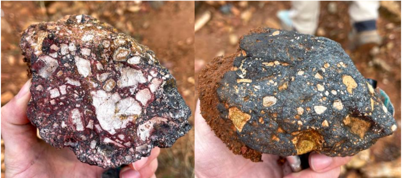
Figure 3. Hematite-Breccia Textures Outcropping at Surface at Morgan's Creek Prospect.
