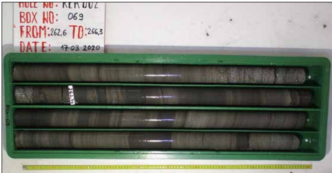
Figure 8-17: Example of the photographic record of core from REK_002 (262.6–266.3 m) Note: The interval 263.15–263.55 m assayed 6.08% B (or 18.6% B 2 O 3 ).
