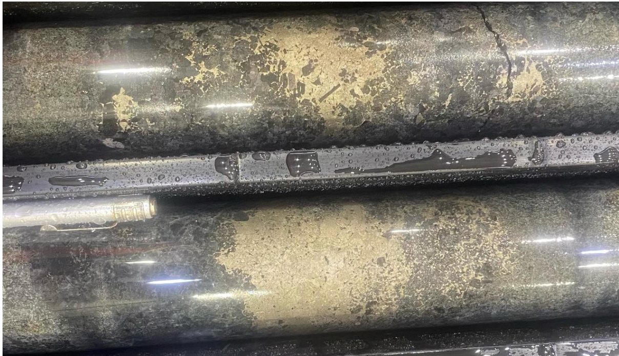
Figure 2: Semi massive 3 phase sulphides in cumulate gabbro-norite, 576.8m
