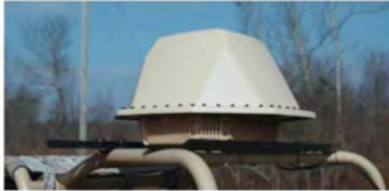
LEFT: A DroneSentry-X C-UAV system mounted on the rollage of an ultra-light tactical vehicle. Image: DroneShield
