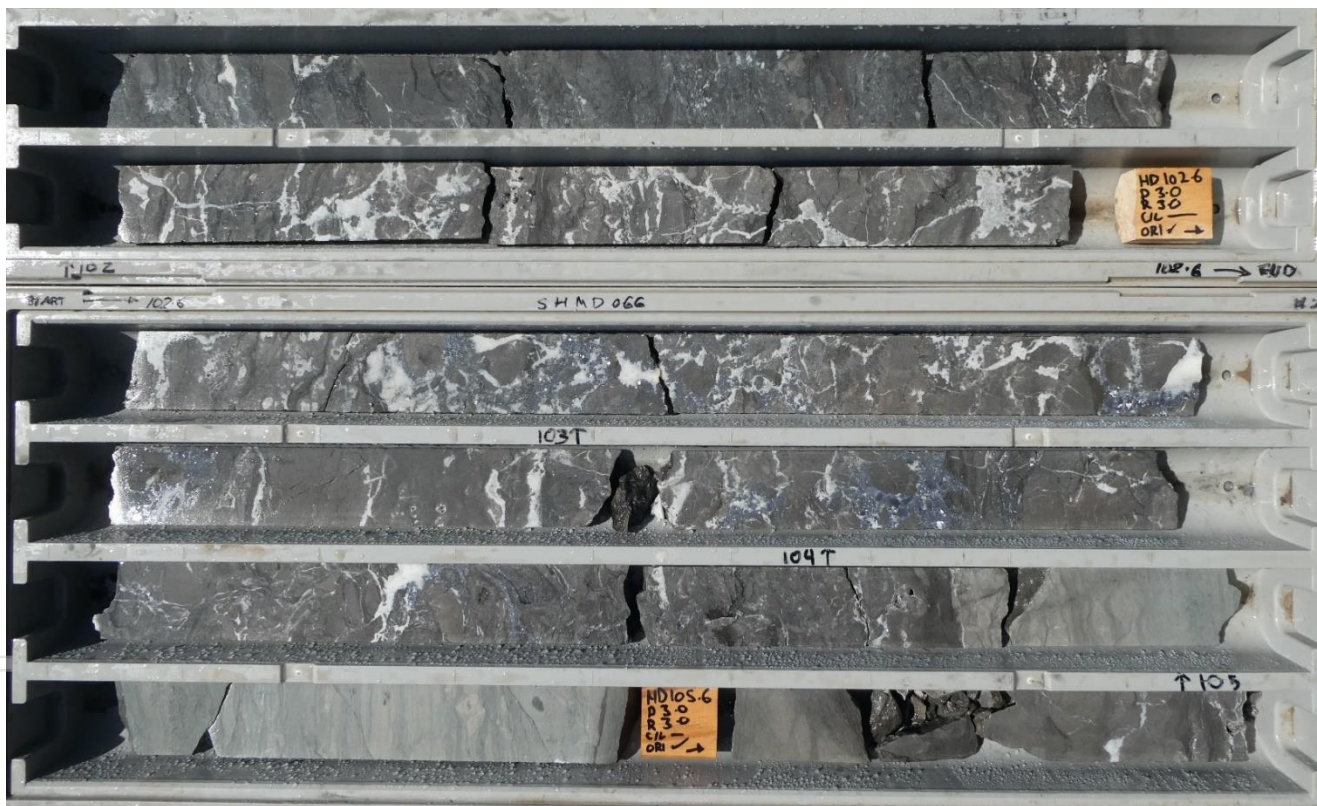
Figure 2 – Core photograph of hydrothermal vein & breccia style of mineralisation intersected in SHMD_066 in NW Omega outside of the current mineralisation envelope.
