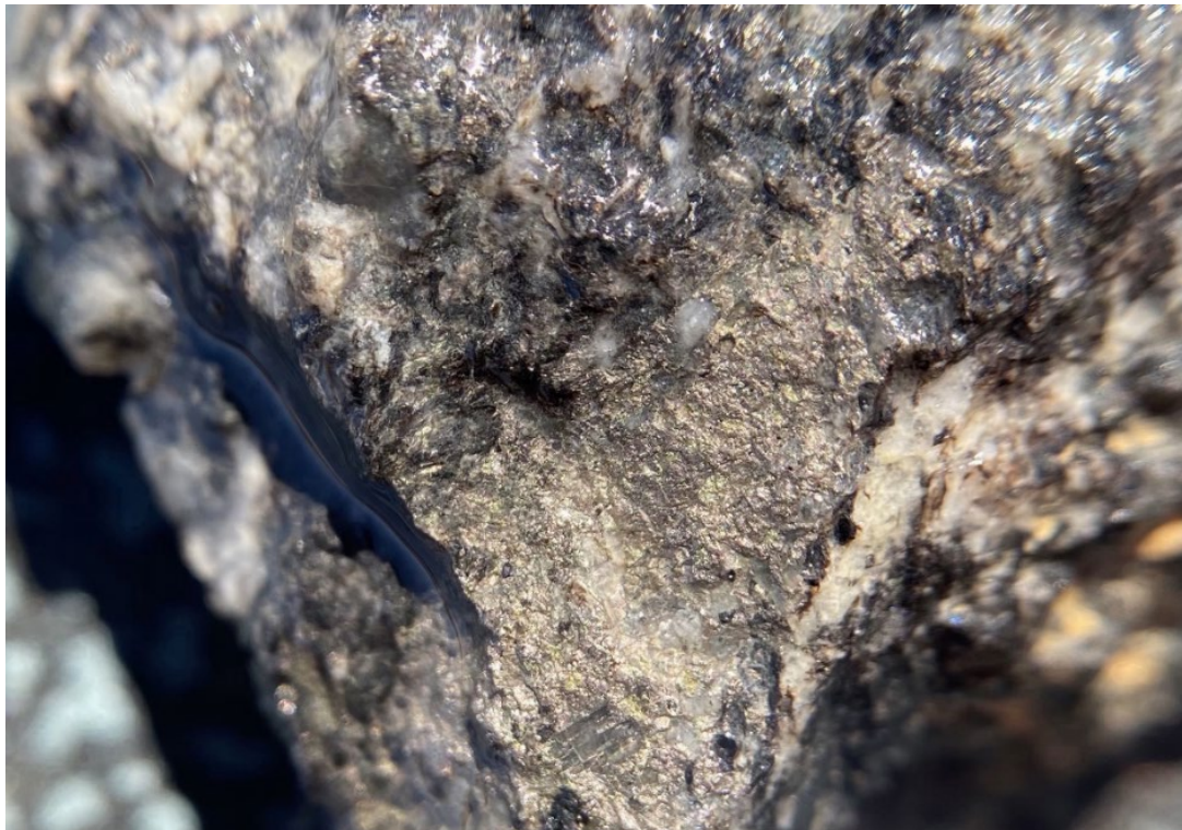
Figure 4 – Photo of a drill chip from PRC009 showing abundant sulphides on a fracture and medium grain texture of the igneous rock (photo colours not altered).
