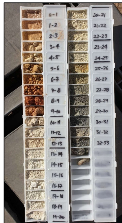
Figure 2: Oar's Gibraltar Project Drill cutting from GBAC069 showing white kaolinitic saprolite developed over gneissic basement material
