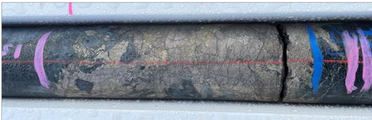
Figure 2. Mineralisation at 156.1m in YAD0017, assaying 4.17g/t PGE (0.95g/t Pd, 3.22g/t Pt), 3.49%Ni & 1.43% Cu.
