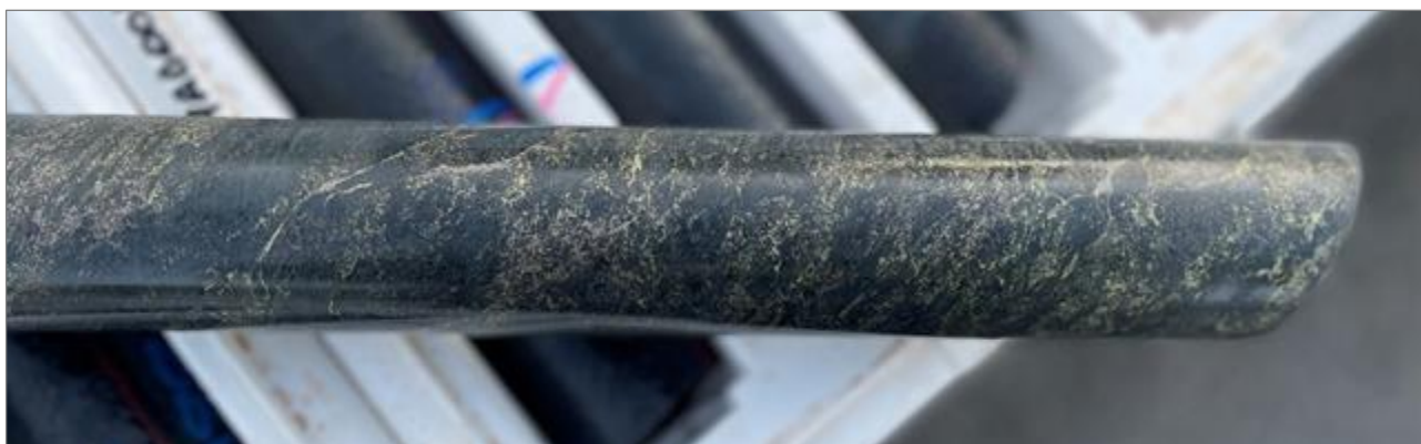
Figure 1. Mineralisation at 308.8m in YAD0017 assaying 4.10g/t PGE (0.77g/t Pd, 3.33g/t Pt), 0.56% Ni & 2.01% Cu.
