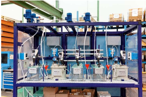
Figure 9 – Single Solvent Extraction Mixer/Settler Circuit
