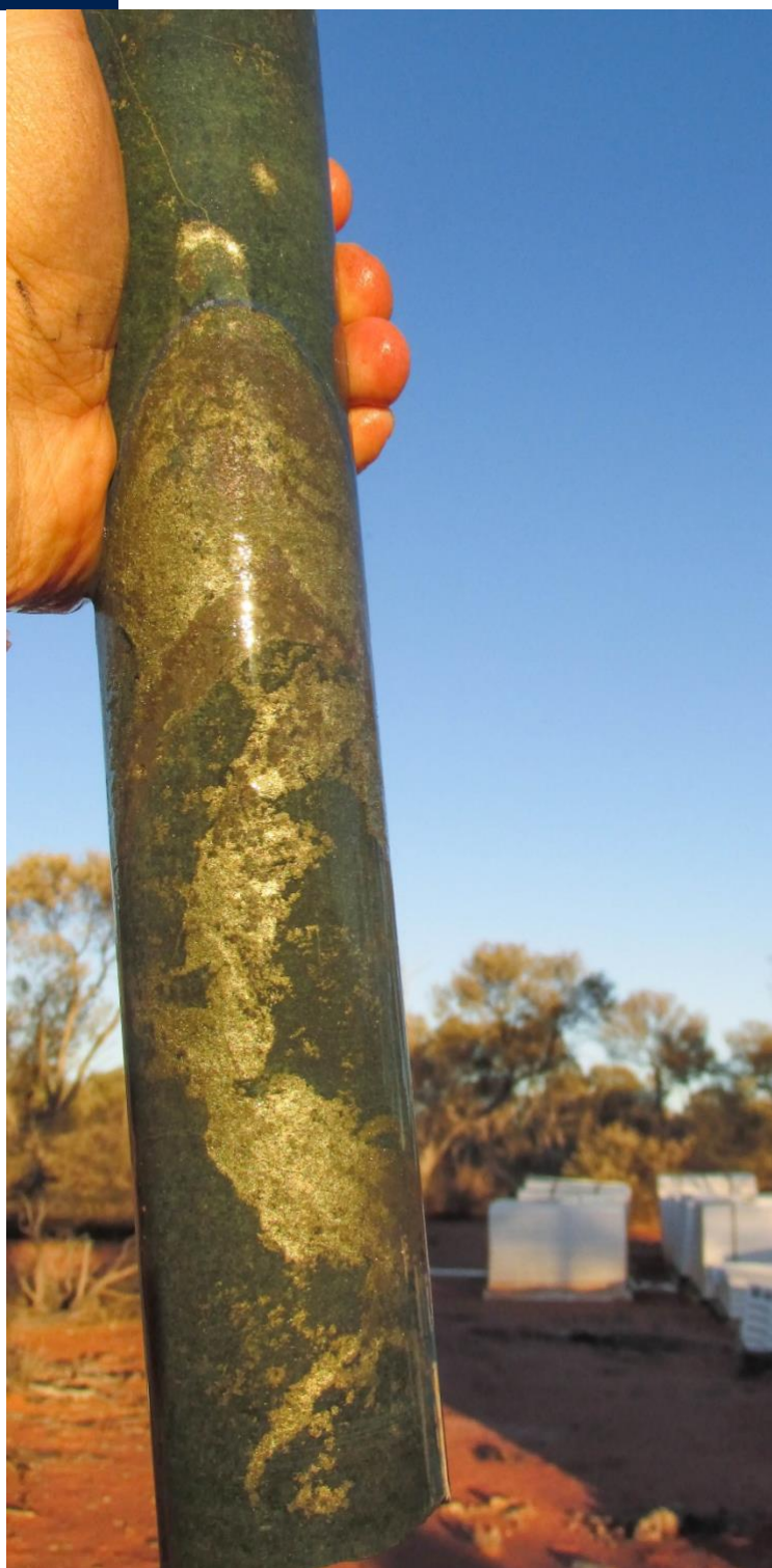
Figure 2: Pentlandite rich stringer sulphides in drillhole DKDD0017
