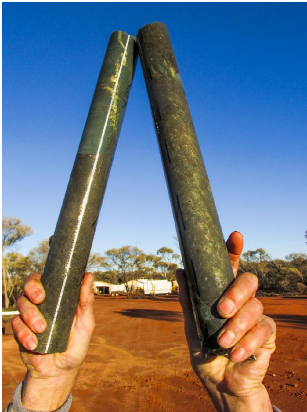
Figure 1: 70cm intersection of massive sulphide in DKDD0017 with the Rosie Camp in the background.
