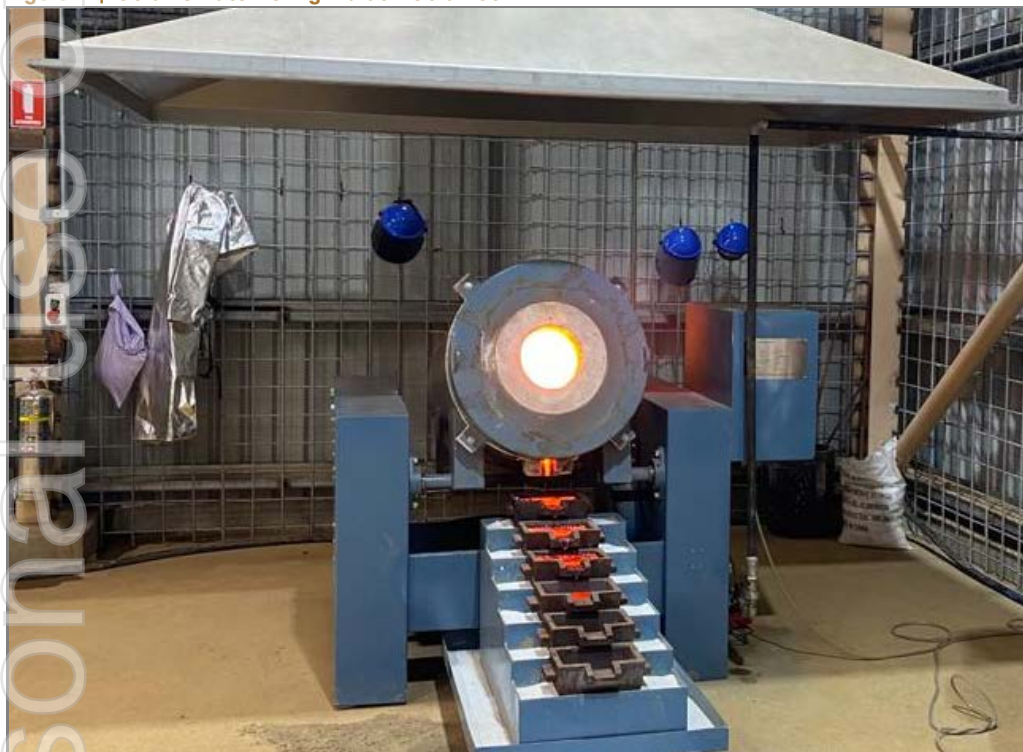
Figure 2 | Gold Furnace During Maiden Gold Pour
