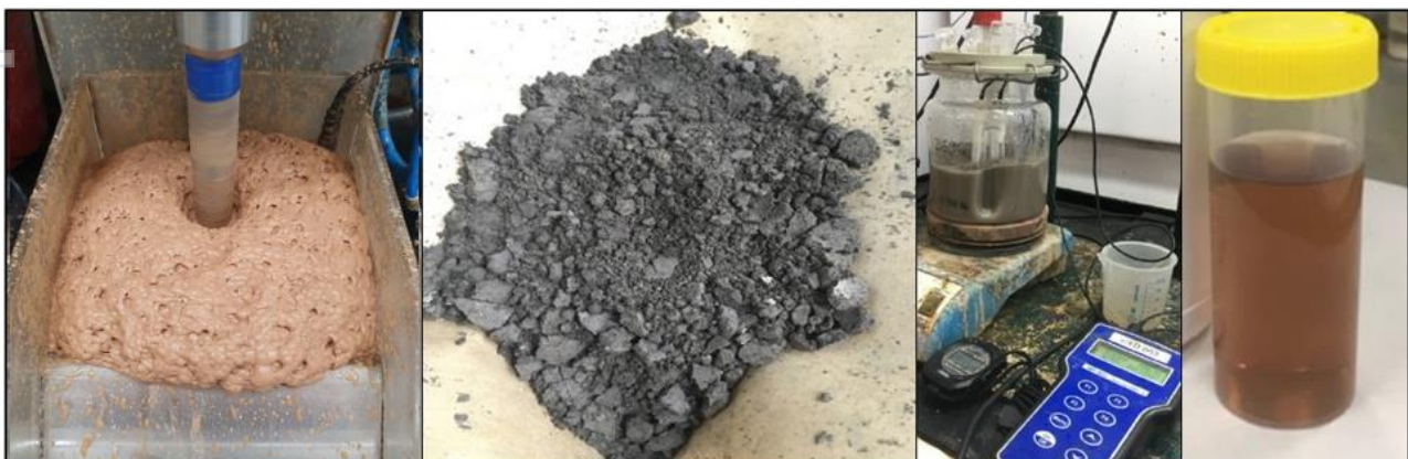
Figure 1 - (L-R) Flotation test, acid bake product, water leach in progress, final water leach liquor.
