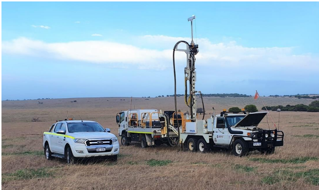
Figure 3 Aircore Resource drilling at the Balline Garnet Project
