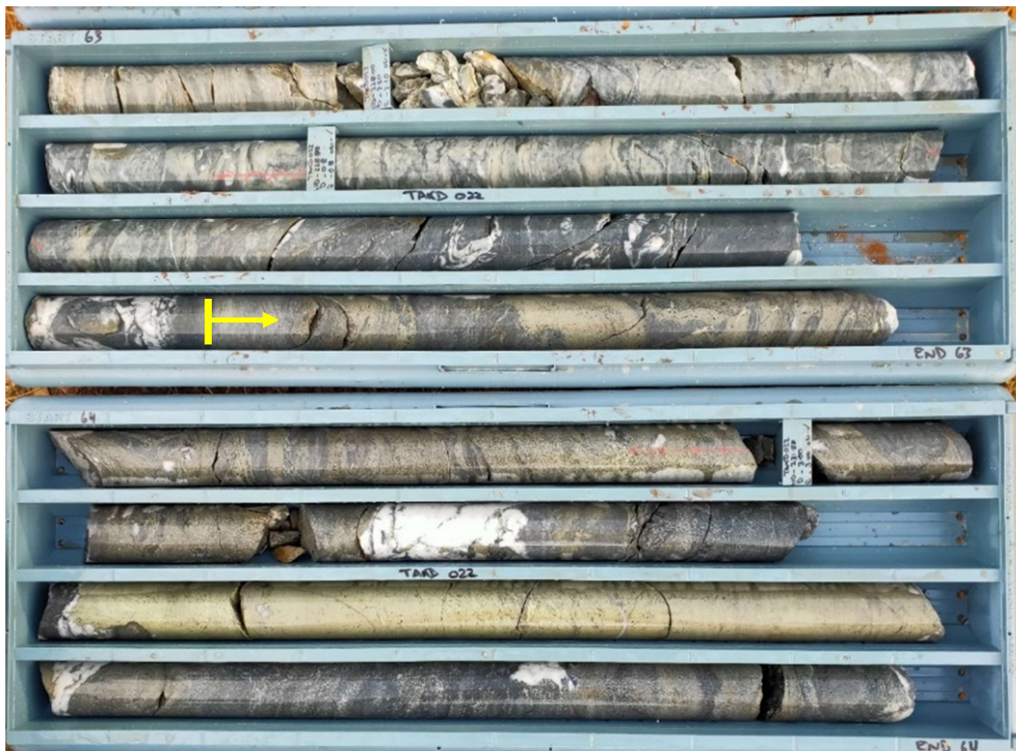
Figure 2 – Drill hole TAKD022 drill core photographs showing the sulphide horizon intersected from 228.6m down hole. Yellow arrows denote the sulphide interval.
