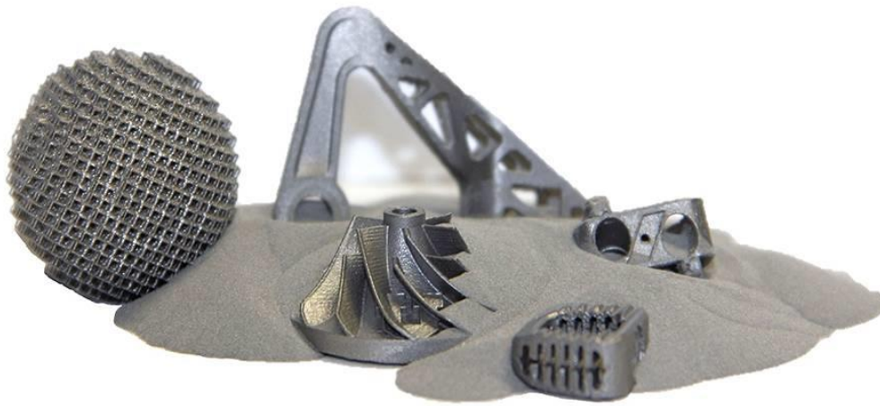
Figure 1: Titanium powder and 3D printed titanium parts
