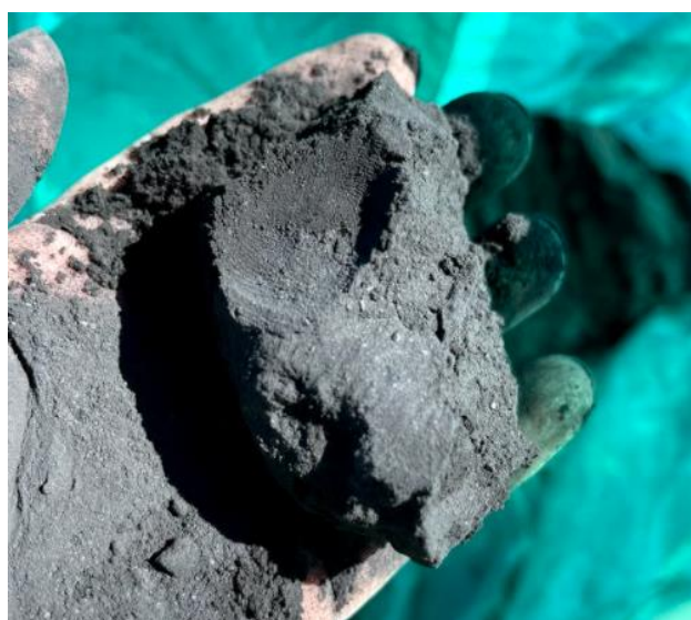
Figure 9 A (left) Rich Chalcopyrite Mineralisation (primary/hypogene zone) from RC Drill Chip from Drillhole WCRC021 (88-89m), which Graded 5.9% Cu , and 9 B (right) Rich Chalcocite Mineralisation in a Black Powder Unit (supergene zone) from Drillhole WCRC006 (18-19m) at Powder Hill, Grading 9.5% Cu .
