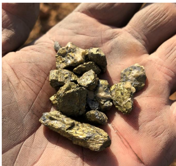
Figure 9 A (left) Rich Chalcopyrite Mineralisation (primary/hypogene zone) from RC Drill Chip from Drillhole WCRC021 (88-89m), which Graded 5.9% Cu , and 9 B (right) Rich Chalcocite Mineralisation in a Black Powder Unit (supergene zone) from Drillhole WCRC006 (18-19m) at Powder Hill, Grading 9.5% Cu .
