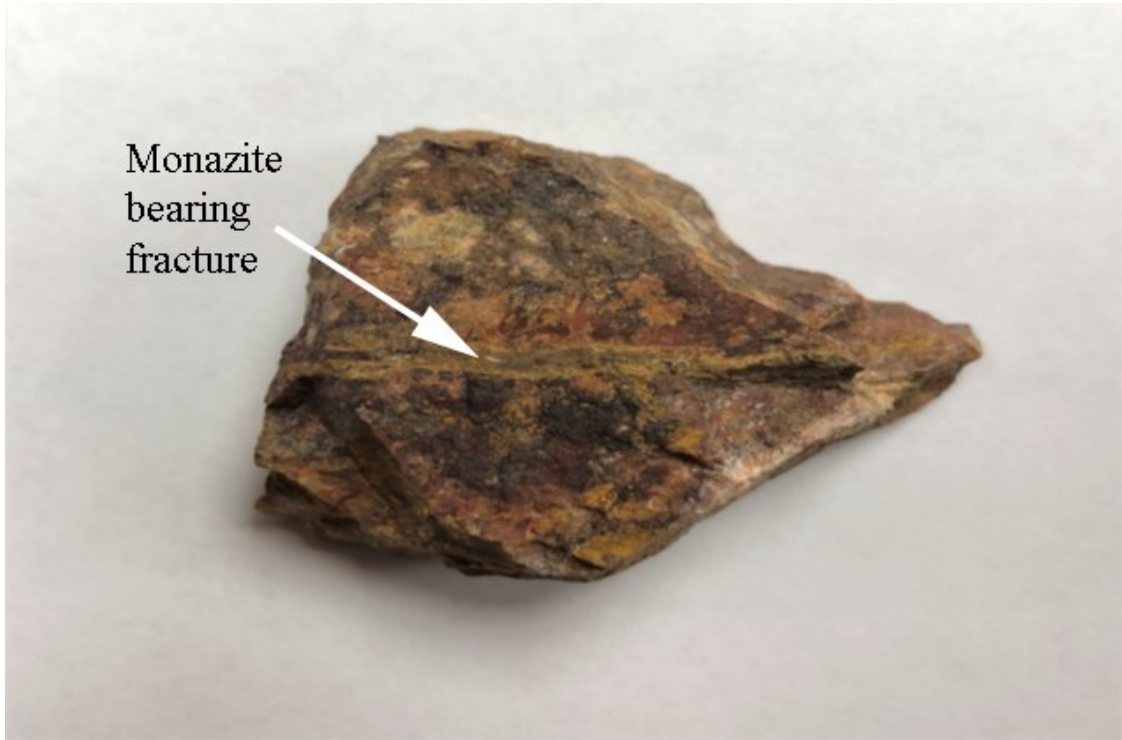
Hand Specimen showing a rusty color and fracture filling
