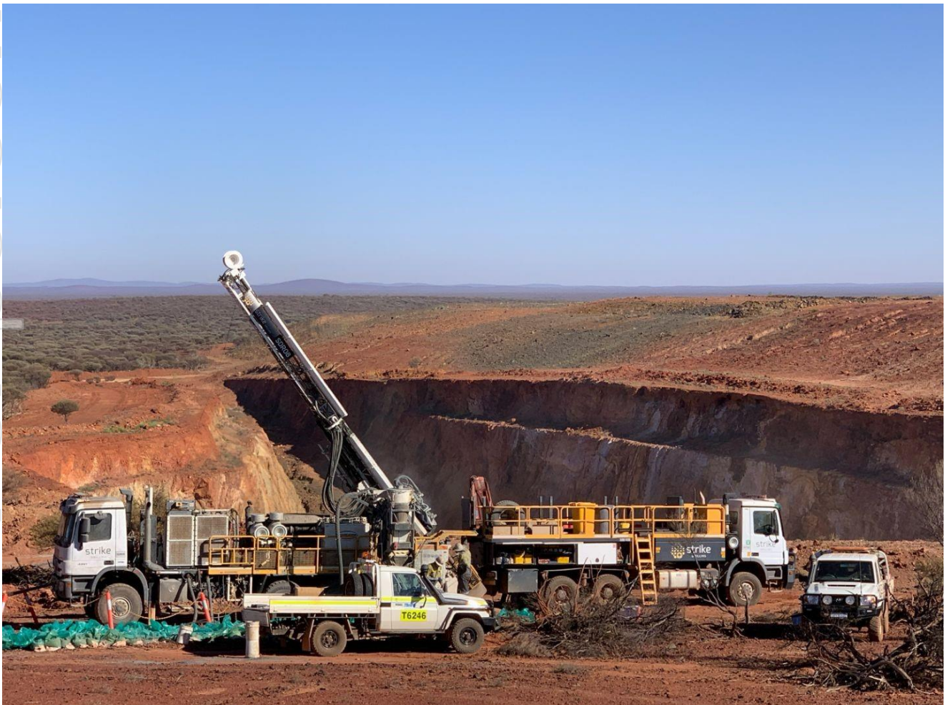
Figure 10. RC drilling activities underway at Bottle Dump.
