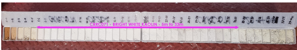
Figure 2: 28m intercept of bright white kaolin in drillhole CRRC071 (5m to 33m)
