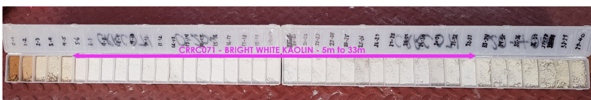
Figure 2: 28m intercept of bright white kaolin in drillhole CRRC071 (5m to 33m)
