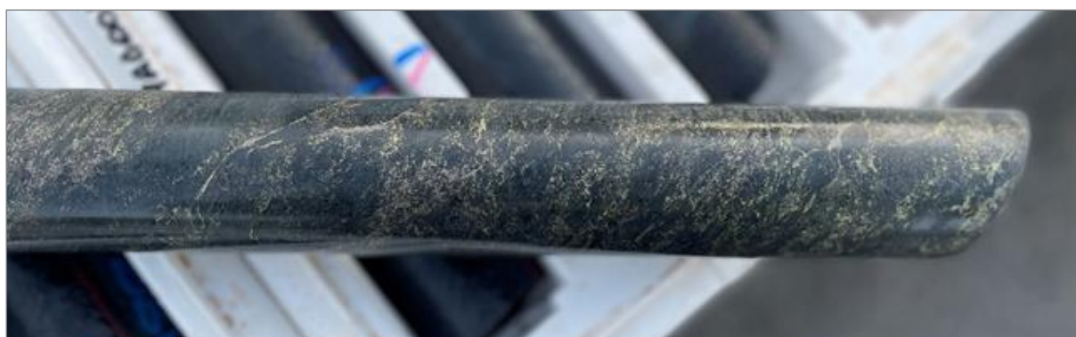
Figure 2. Disseminated to stringer chalcopyrite-rich sulphides at 308.8m in YAD0017.
