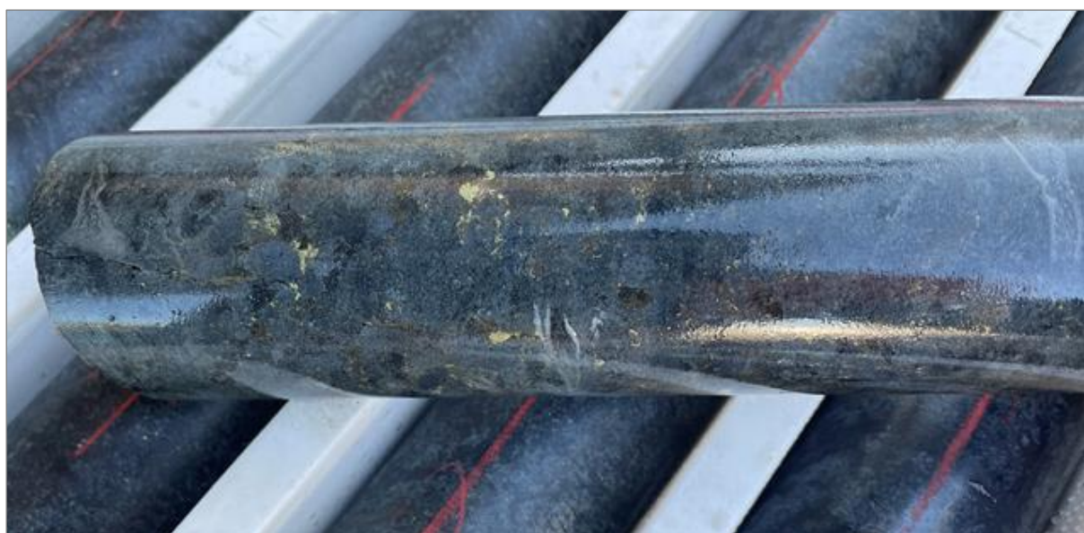
Figure 6. Disseminated blebby chalcopyrite at 161.8m in YAD0018.
