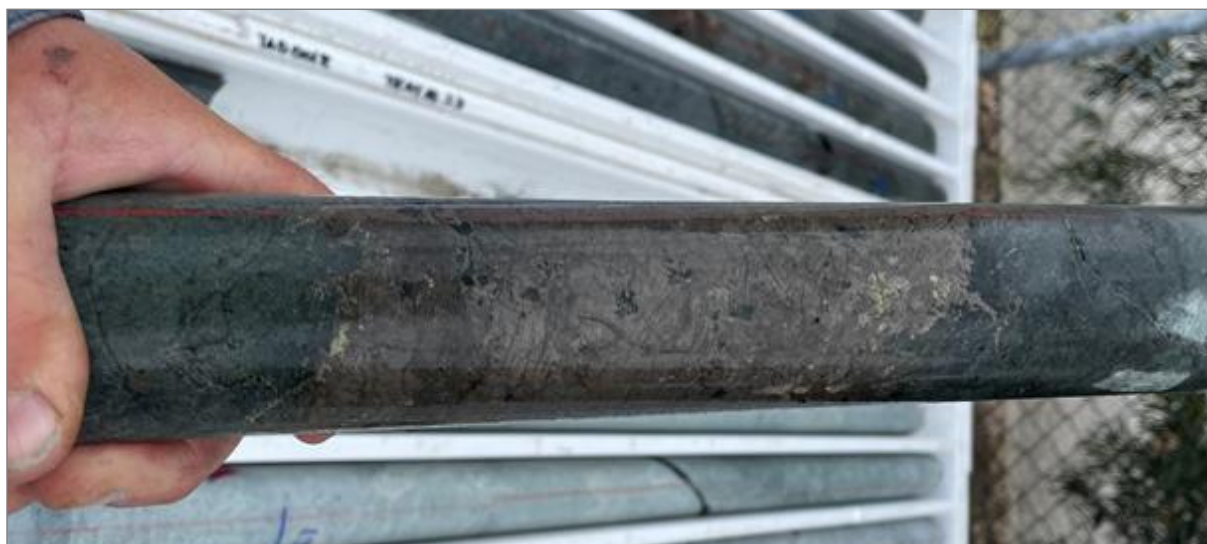
Figure 5. 20cm zone of massive sulphide at 130.8m in YAD0018.
