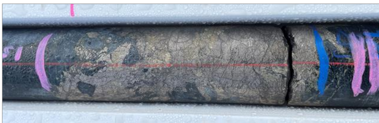
Figure 4. 20cm of massive sulphide at 156.1m in YAD0017.
