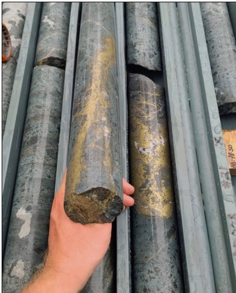
Figure 7: Chalcopyrite vein in intensely chlorite and silica altered unit with zones of strong brecciation and disseminated microsulphide throughout groundmass, MCDDH008.
