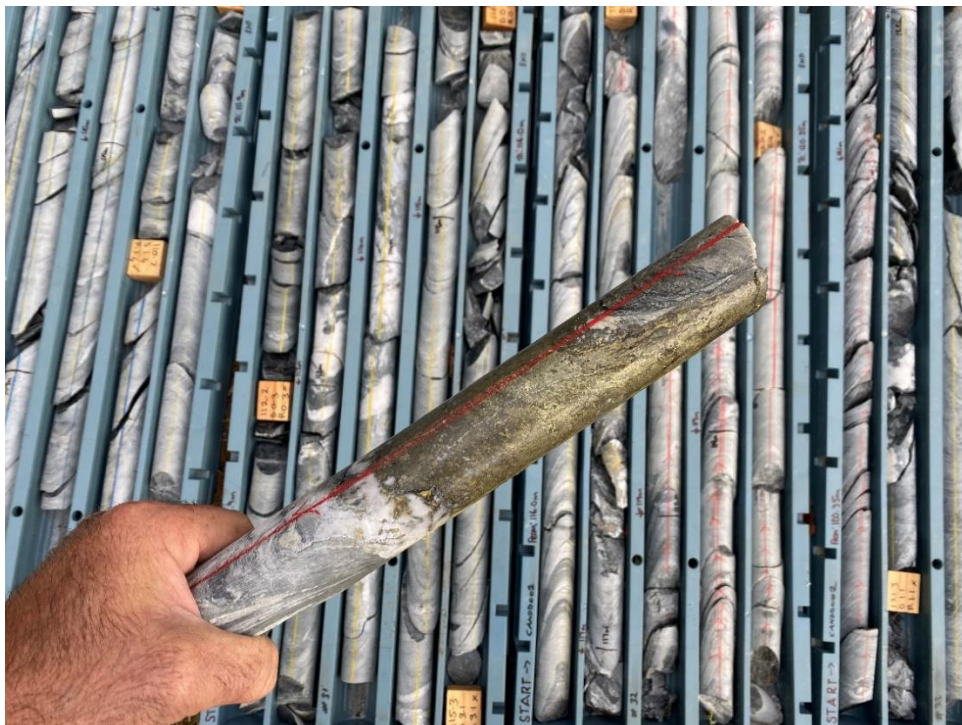
Figure 2: Example of copper bearing sulphide (chalcopyrite) veins (at 118 metres) in a new copper zone intersected higher in CANDD002.
