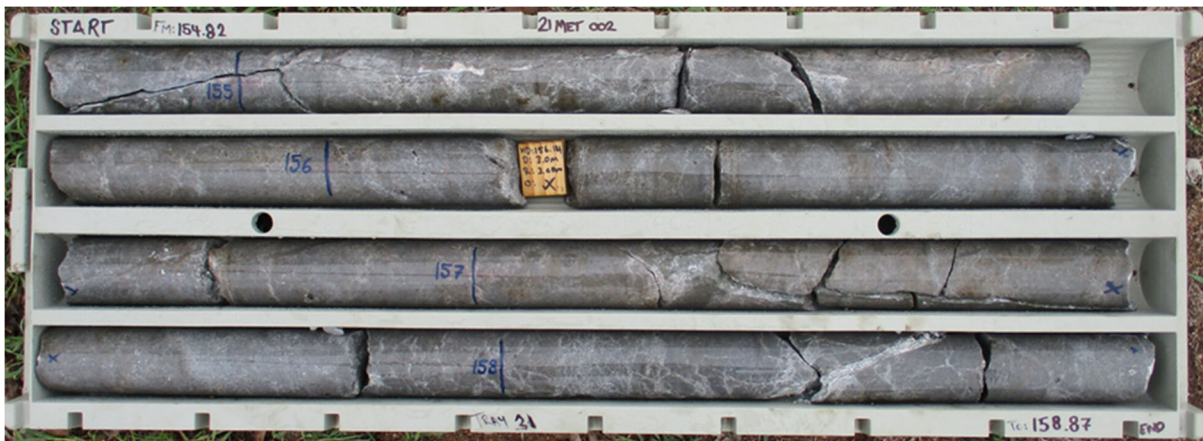
Plate 2-South West Slopes Vuggy Silica Alteration, with very fine-grained disseminated sulphides
