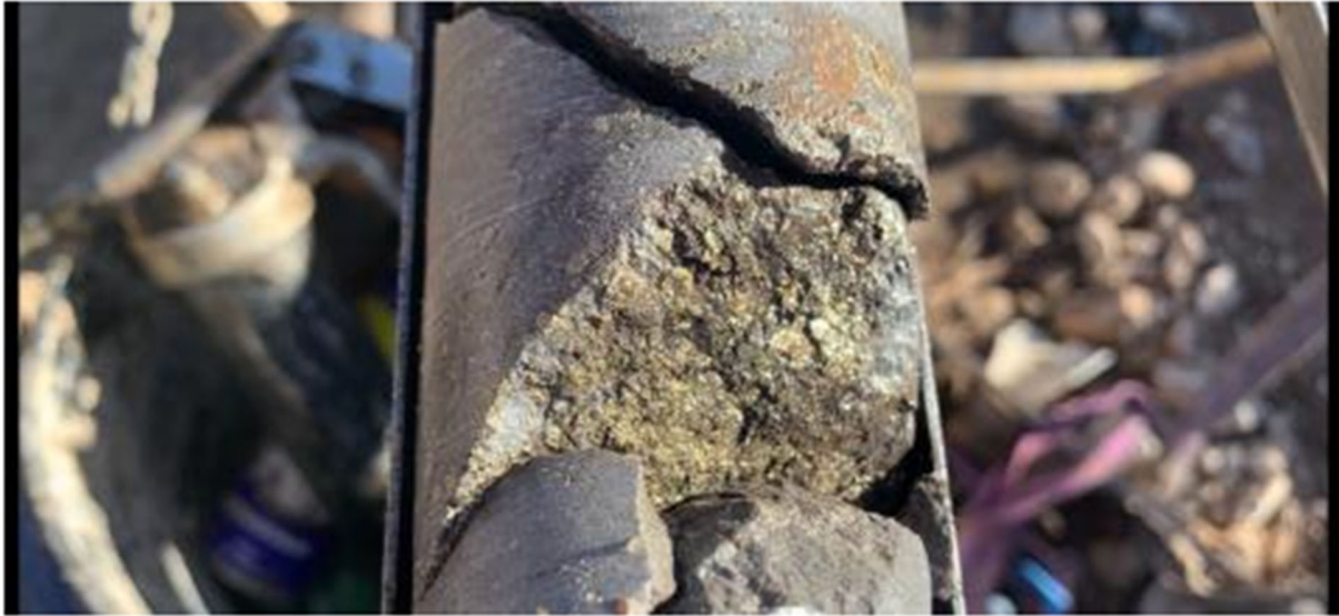
Plate 1- South West Slopes Sulphide Mineralisation (MET001 @ 127m depth)
