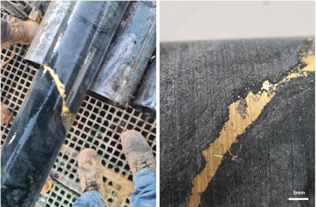
Figure 1. Significant visible gold in the NQ diamond drill & a close-up of the gold seam
