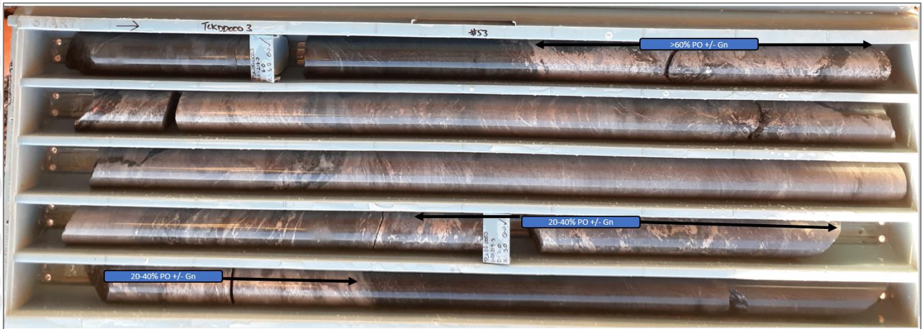
Figure 4. Diamond core from TCKDD003 showing sulphide-rich BIF unit from 216 to 220m.
