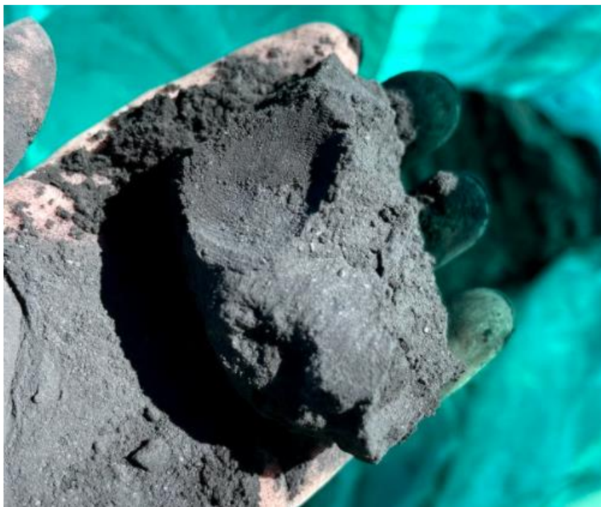
Figure 2. Rich Chalcocite Mineralisation in a Black Powder Unit (supergene zone) from Drill Hole WCRC006 (18-19m) at Powder Hill, Grading 9.5% Cu .
