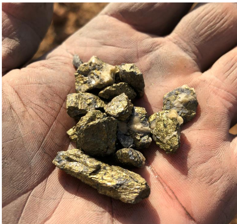
Figure 1. Rich Chalcopyrite Mineralisation (primary/hypogene zone) from RC Drill Chip From Drillhole WCRC021, from the 88-89m Intercept which Graded 5.9% Cu Within a Broader Intercept of 11m @ 1.5% Cu .
