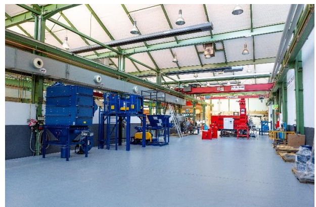
Figure 6 – Render of DP in Hilchenbach showing battery shredding (left, foreground) and hydrometallurgical refining circuits (right, background)
