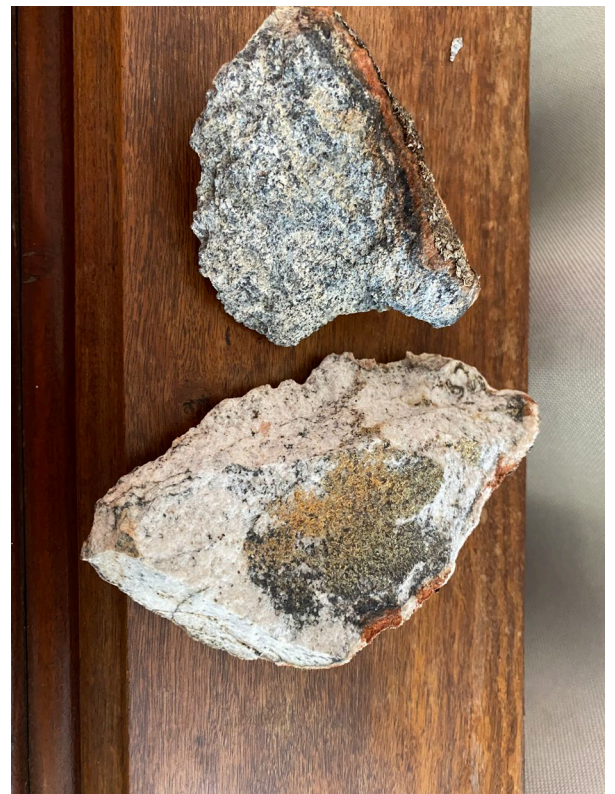
pXRF sampling at West Emu and the speckled ultramafic beside the white felsic intrusive rock
