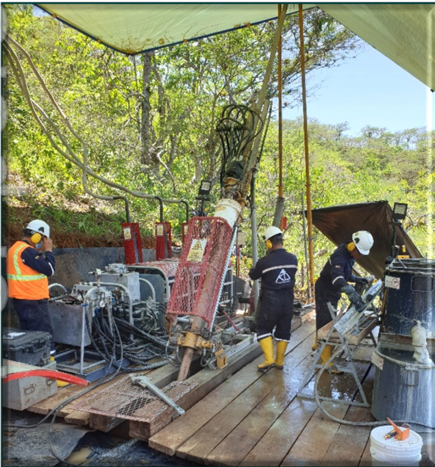
Figure 3: Diamond drill platform at Papayal padsite TPD001
