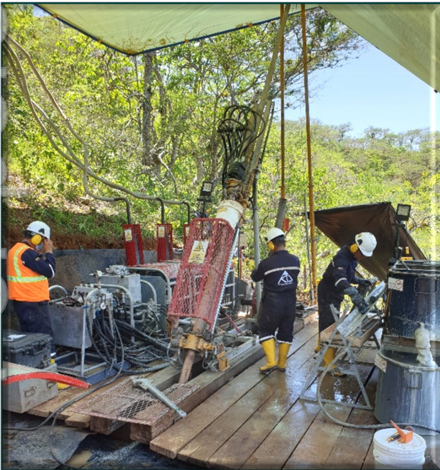
Figure 3: Diamond drill platform at Papayal padsite TPD001
