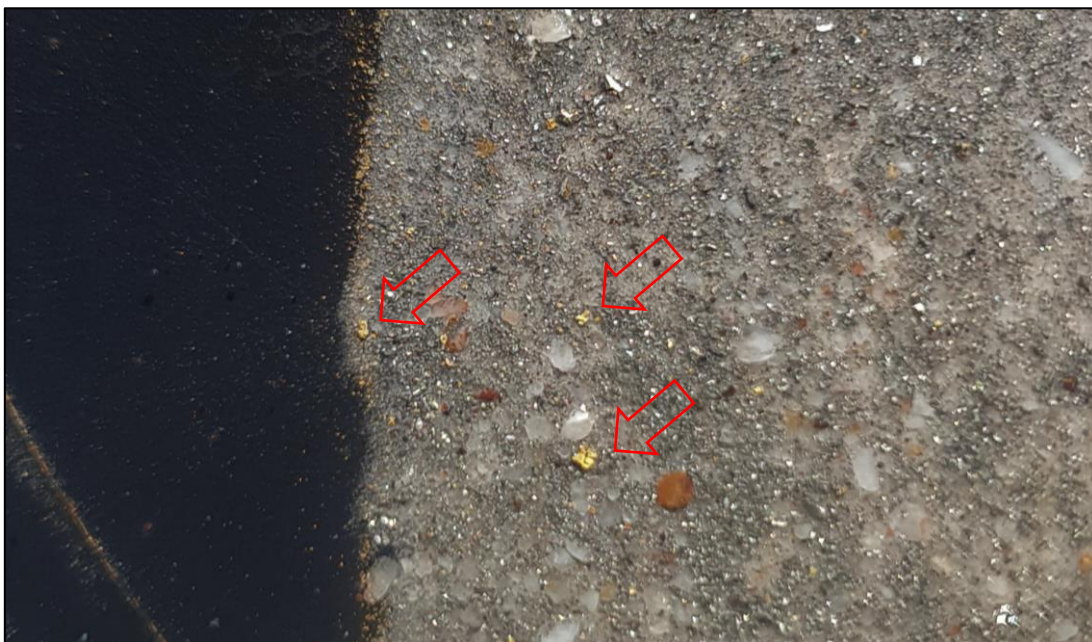
Figure 3. Photo of small gold nuggets recovered from panned concentrates in sample number NMRMW-BS028. The presence of small nuggets demonstrates to NMR that the area is “nuggety” in its style of mineralisation and that the gold is accessible using simple gravity separation techniques. A few of the many small nuggets are highlighted in the photo above. Additional fine gold can be seen distributed along the left-hand edge of the panned concentrates.
