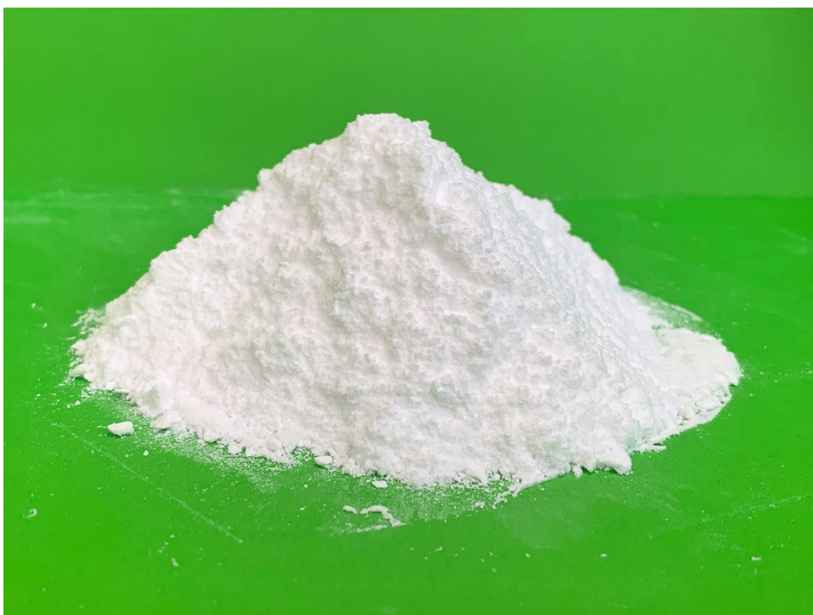
Figure 5: Primary Lithium Sulphate produced under metallurgical testing for AVZ's planned Manono Lithium Sulphate Plant
