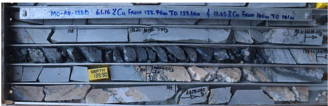
Figure 1: High grade vein hosted bornite/chalcocite mineralisation including an interval of 61.16% Cu from 138.70m to 139.60m downhole depth intersected in hole MO-A4-138D at A4 (refer ASX Announcement dated 1 December 2020).
