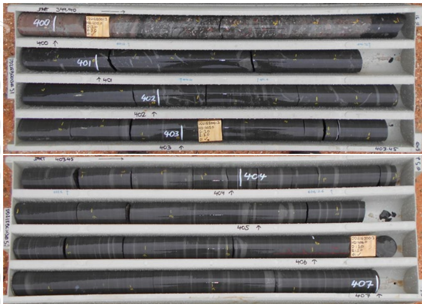
Figure 6 Core photos showing the upper contact of the Tapley Hill Formation in hole DD21EB0013. Mineralisation is fine grained and largely non-visual at this scale.
