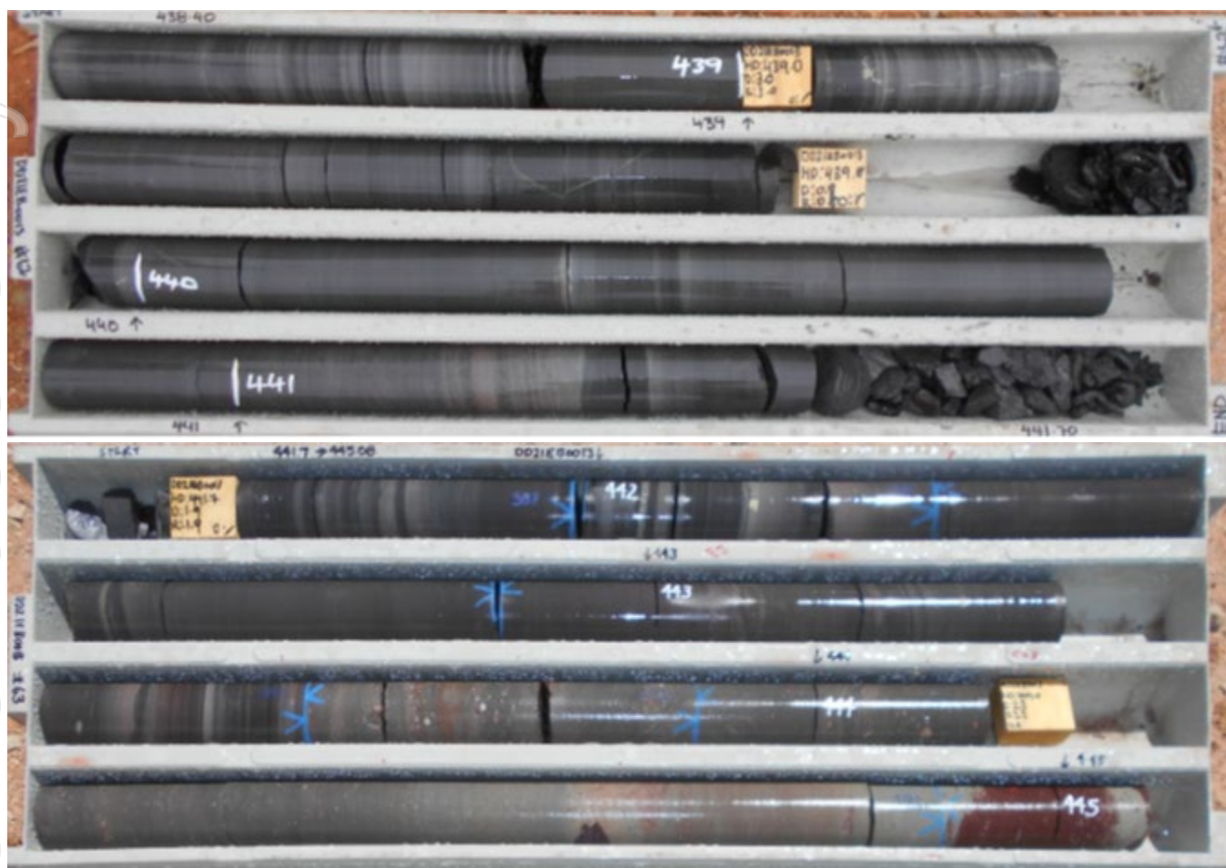
Figure 7 Core photos showing the mineralised lower contact between Taply Hill Fm shale and Pandurra Fm in hole DD21EB0013.
