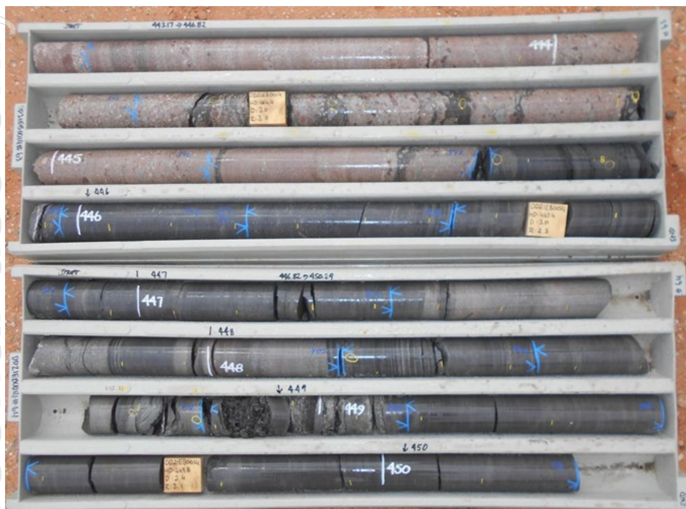
Figure 8 Core photos showing the mineralised upper Tapley Hill Fm shale contact with Whyalal Sandstone in hole DD21EB0014. This hole is located near the eastern edge of the shale body; as the Tapley thins out to the east, mineralisation is anticipated to become more intense.
