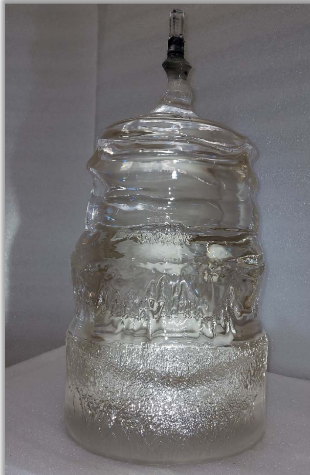
~90kg single crystal sapphire glass boule grown by ALOX using Alpha’s HPA pellet feedstock
