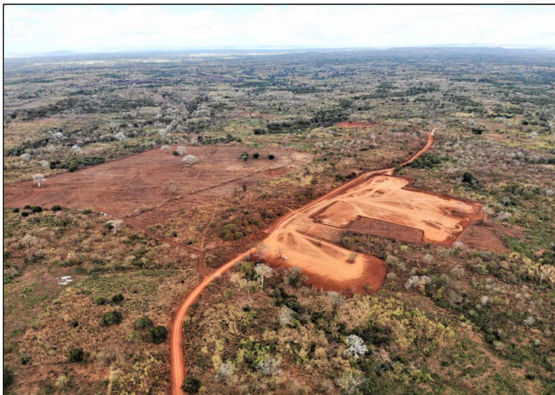
Figure 3: Aerial view from the southwest of the earthworks completed including the ROM and Processing Plant area in the foreground and clearing for the TSF area directly towards the north.
