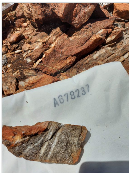
Figure 11: Sampled stockwork veining hosted by highly sheared mafic intrusive and surface expression of a northerly trending regional fault zone that cross cuts the mafic intrusive unit
