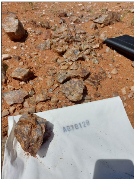
Figure 9: Sampled quartz veining and quartz veining hosted in shear zones
