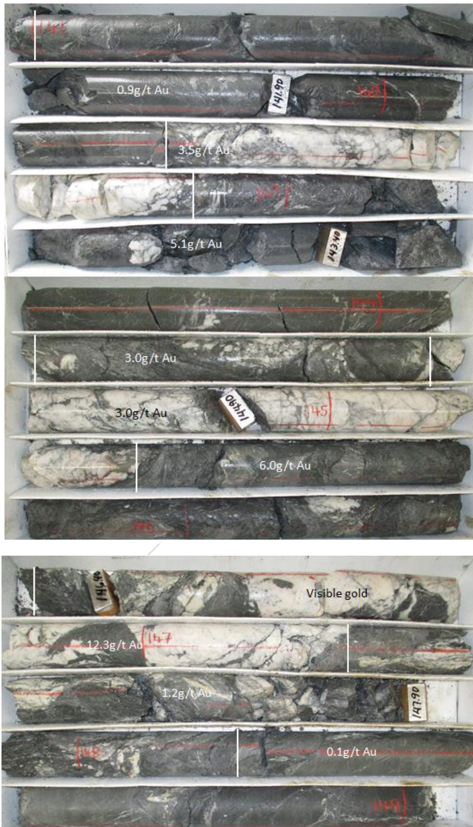
Figure 13. Quartz reef intersected in Big River hole BRDDH027 with gold assay results between 142m and 148m. Visible gold occurs at 146.7m.
