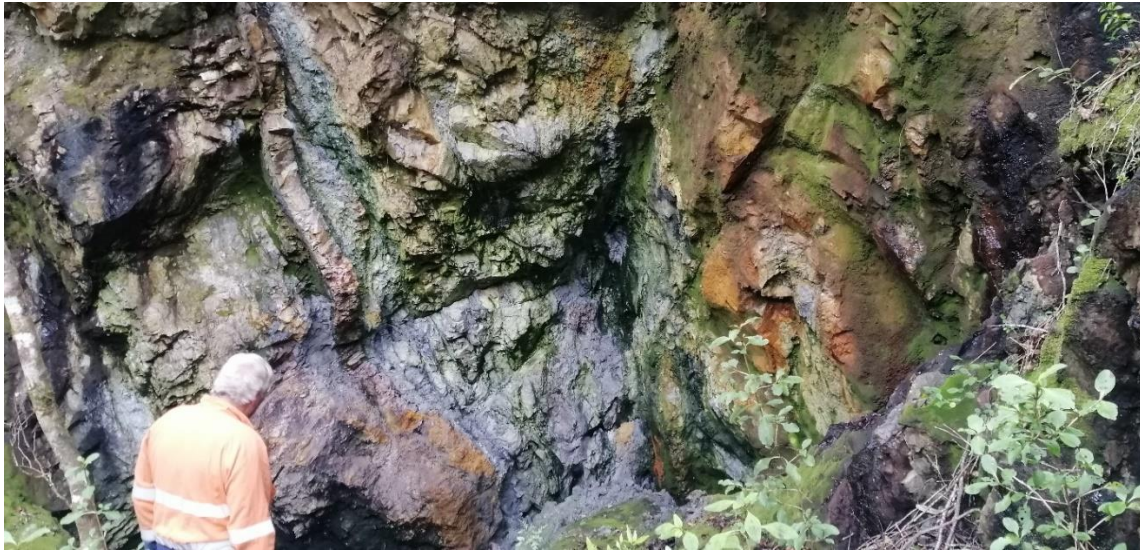
Figure 8. A2 quartz reef between dotted white lines ~1m thick surrounded by sulphide rich sediments.
