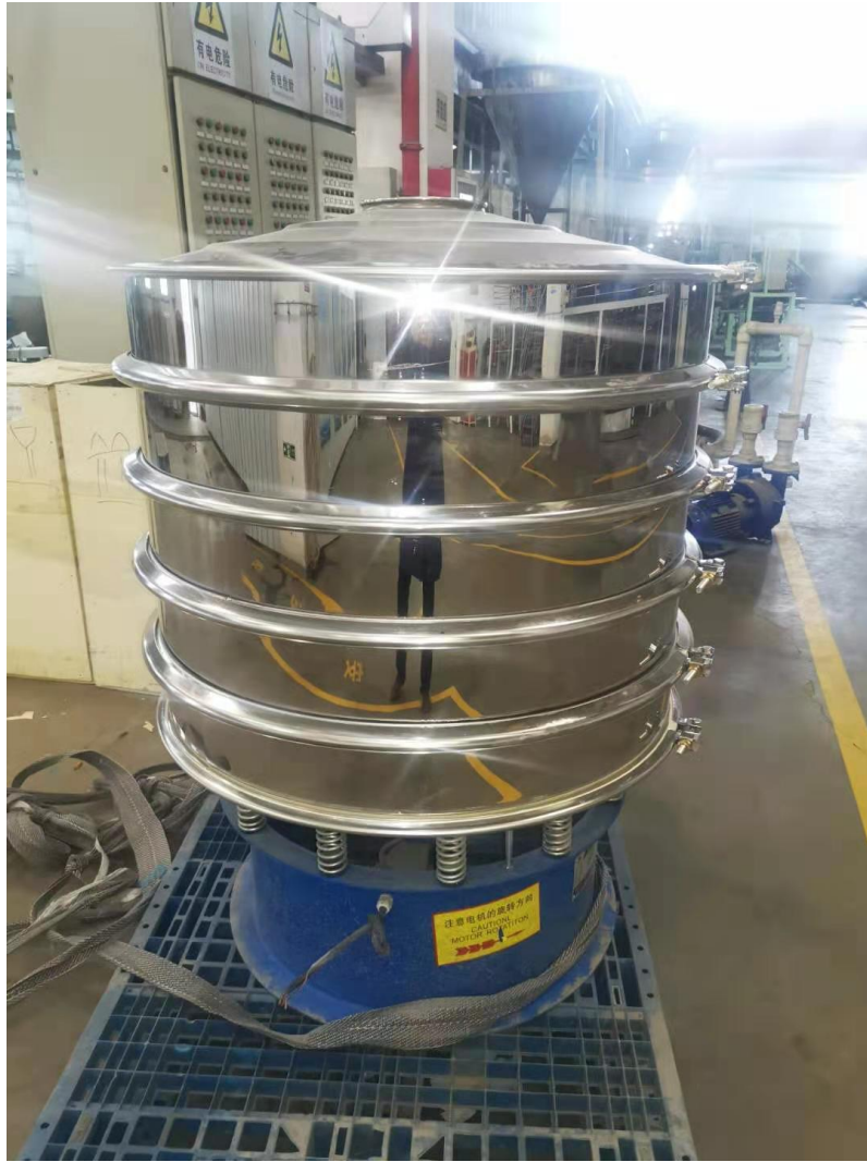
Figure 2 – Vibrating screen used at testing facility
