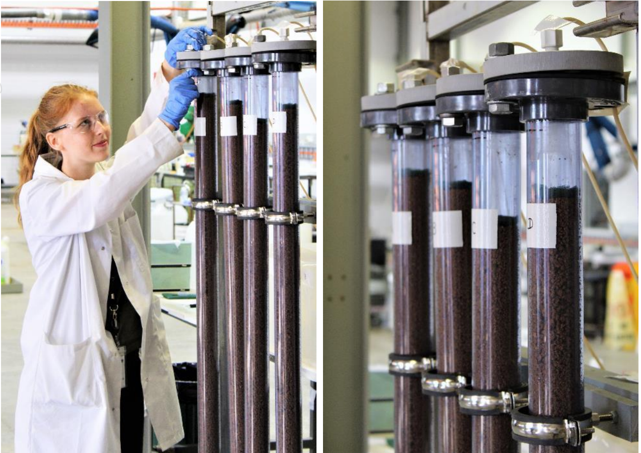
Figure 1: Heap leach columns under desorption (irrigation) at ANSTO Minerals in Sydney.
