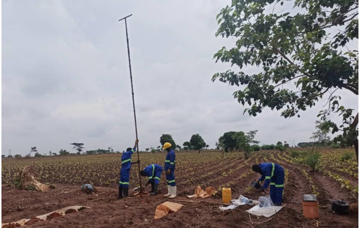
Figure 3. Sovereign’s field team hand-auger drilling at Nsaru.
