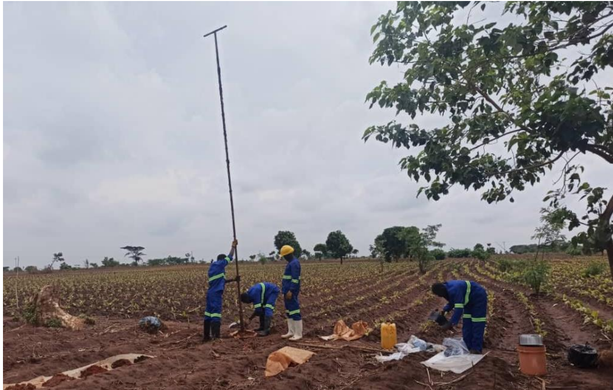
Figure 3. Sovereign's field team hand-auger drilling at Nsaru.
