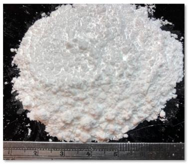
Batch 6 HPA powder product (>99.99% Al<sub>2</sub>O<sub>3</sub>) produced from an industrial chemical feedstock
