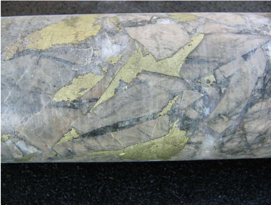
Fig 4. Mt Cannindah Mineralization Style : Breccia Infill in metasediments: QMCMD022, 260.00m. Infill Breccia, chalcopyrite-pyrite. Qld Ores core photo – 2008 report.
