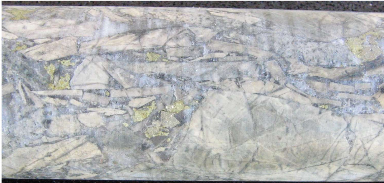
Fig 5. Mt Cannindah Mineralization Style : Breccia Infill in metasediments.(QMCMD022). 'Splinter' breccia. The 'splinter' breccia was probably produced by fluid pressure cracking an overpressurised carapace. Dilational structures have acted as conduits for ore fluids from a potential stock at depth. Qld Ores core photo – 2008 report.
