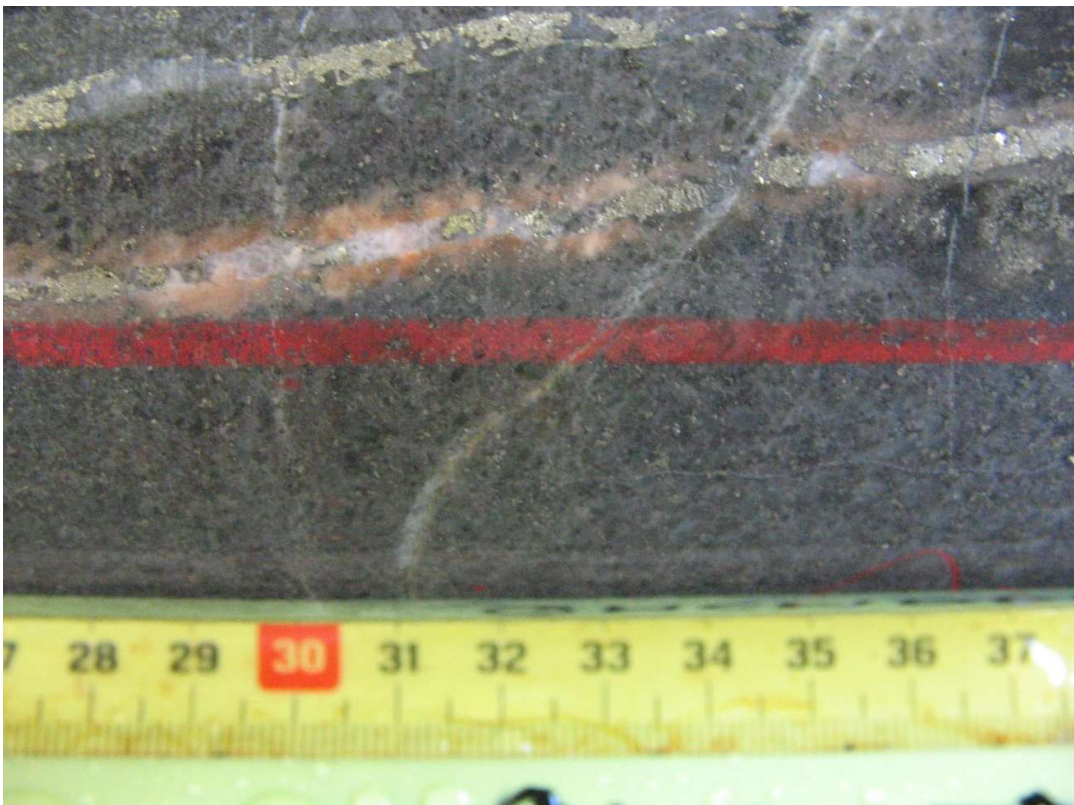
Fig 9. Mt Cannindah Mineralization Style Intrusive hosted Vein & Disseminations .QMCMD025, 162.50m. 1mm wide pyrite-quartz -carbonate-chlorite-chalcopyrite veins with pink K-feldspar selvages. This early vein event, overprints early alteration of the Cannindah Intrusive, followed by later mineralization events. Qld Ores core photo – 2008 report.
