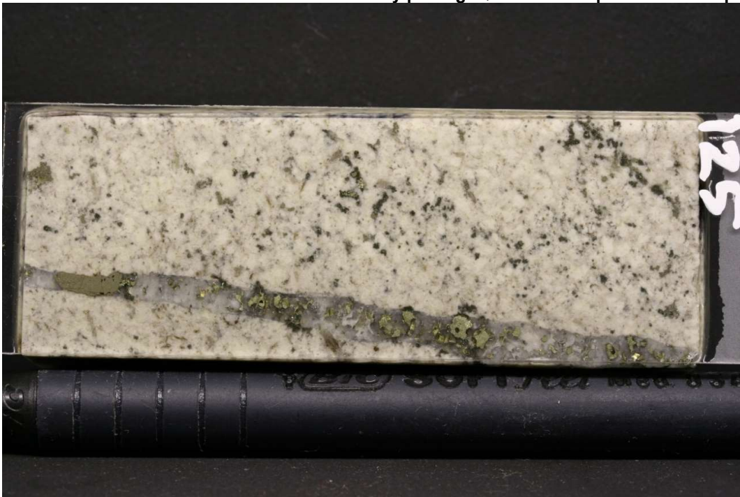
Fig 7. Mt Cannindah Mineralization Style Intrusive hosted Vein. QMCMDD010, 125.20m. Sericite-carbonate altered diorite with chalcopyrite and pyrite, both disseminated and in veins. Qld Ores core photo.
